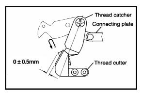
check the standby position of the thread catcher. (Fig.5)
