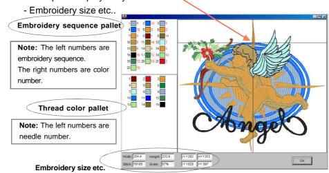
\*Although the needle numbers are automatically selected, they can be changed by dragging a color from thread color pallet to the embroidery sequence pallet.
