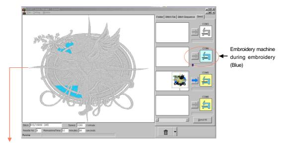
\*On the monitor screen, the progress of the embroidery can be checked both with simulation and numerical value.
