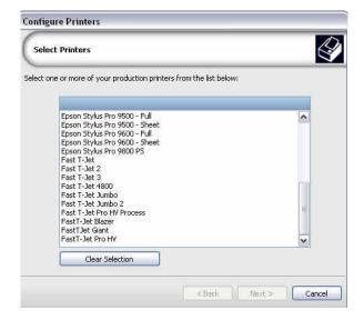
The second window will ask for the **printer package**. A printer package contains all of the custom **Print Modes** that tell FastRIP how to print on garments. Your version of FastARTIST may automatically install these print modes and printer packages.
