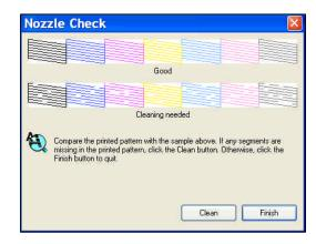
Note: For serious clogs you can run this routine several times or install the refillable cleaning cartridges and run several head cleanings.
