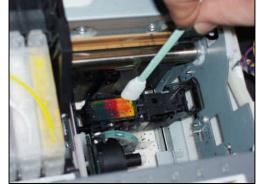
The pictures on the right show two very dirty capping stations. The capping station seals the print head when it is not in use. Ink residue around the edge of the capping station keeps the head from seating and sealing properly which can cause head clogs. White ink will buildup a little more than normal colors.
