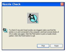
**5.** After the *Nozzle Check Pattern* has printed out check to see if the lines have any gaps or lines in them. If the *Nozzle Check Pattern* has no gaps or lines click *Finish*.
