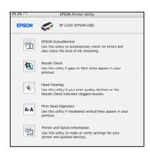
You should never turn off the printer while the power light is flashing, this may damage the printer. You can do head cleanings at any time even when the printer is printing. It will stop and clean the heads and resume right where it left off. Since the Head Cleaning cycle also wipes the bottom of the head, it is recommend to do head cleanings if you start to see drops of ink on garments or if the head comes in contact with a garment.
